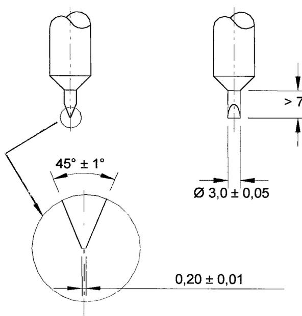
NOTE 1 All dimensions with a tolerance are machined as EN ISO 1302 [9] to  $\sqrt{Ra\ 0,4}$
