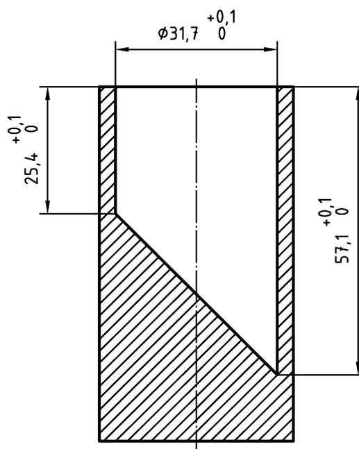
Figure 4 — Small parts cylinder
